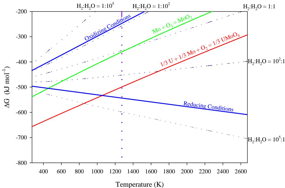
Figure 7: Ellingham diagram illustrating the range of  $p\text{O}_2$  to be tested and the change in  $\Delta G$  for the formation of  $\text{MoO}_2$  and  $\text{UMo}_6$ [6]
