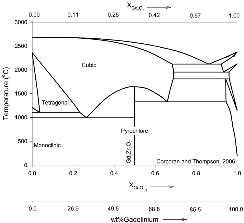
**Figure 1: ZrO<sub>2</sub>-Gd<sub>2</sub>O<sub>3</sub> Binary Phase Diagram**
