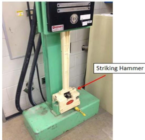
Figure 1-Charpy impact testing apparatus.
