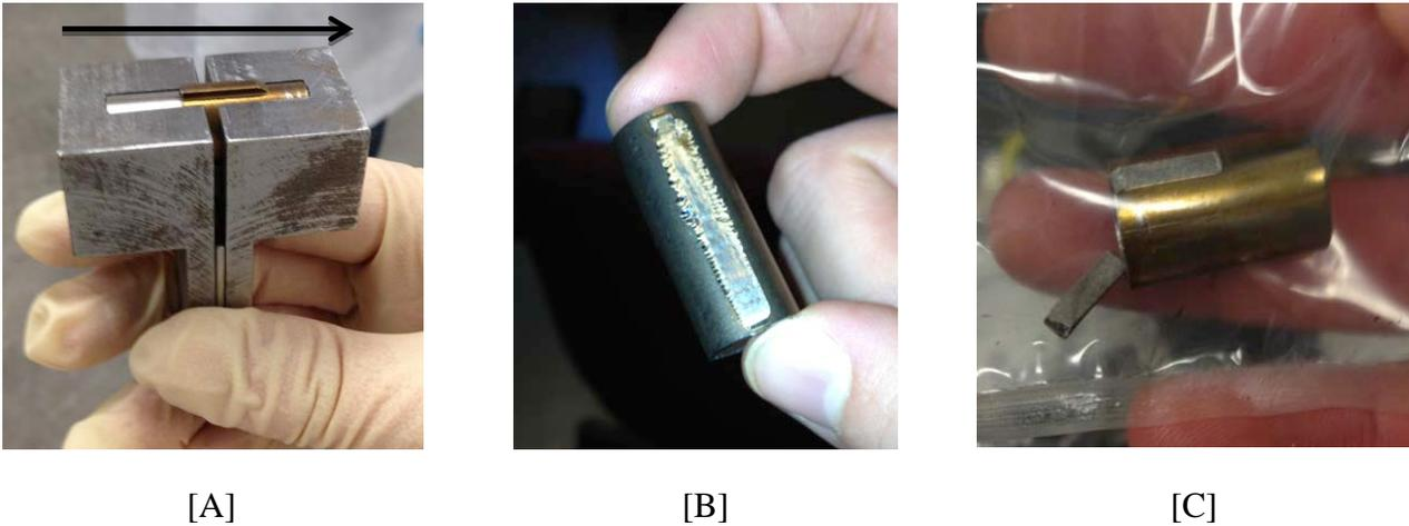
Figure 2-[A] Half-length sample in a specialized jig (arrow indicates direction of striking hammer motion), [B] Deformed full bearing pad from an unsuccessful impact test, [C] Fractured bearing pad joint from a successful impact test.
