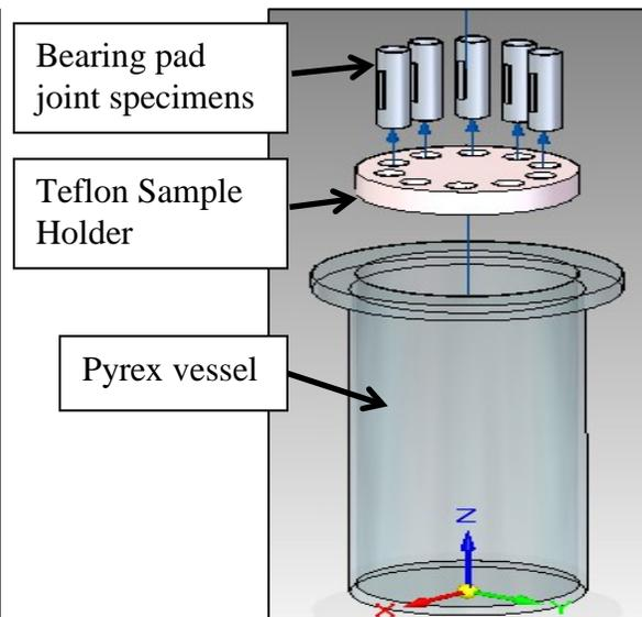
Figure 3- Exploded view of the test apparatus, showing the glass vessel, Teflon sample holder, and brazed bearing pad specimens.
