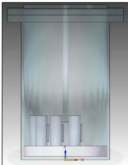
Figure 2- CAD model of the corrosion test apparatus.
