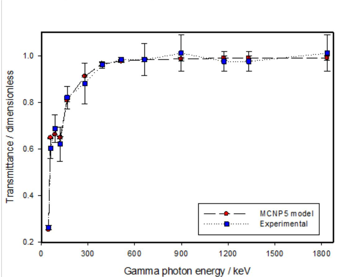
Figure 6: Experimental and MCNP5 transmittance results for a single layer of the second generation CRC fabric [13]
