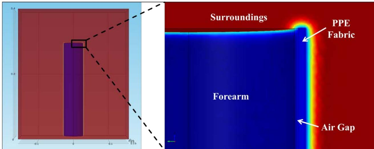
Figure 2: Preliminary particulate transport model developed using the COMSOL Multiphysics software (red and blue areas represent regions of high and low concentration respectively)
