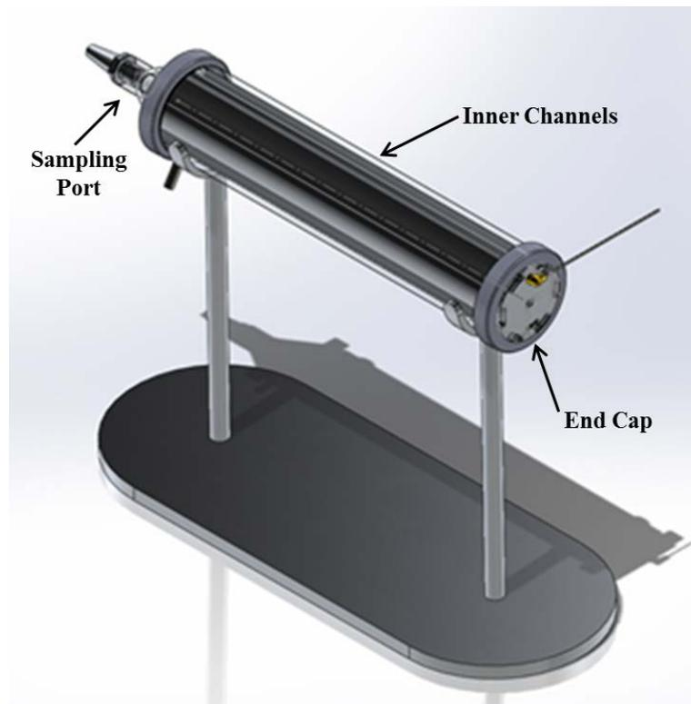
Figure 4: Phantom forearm apparatus used for the particulate transport benchmarking experimentation
