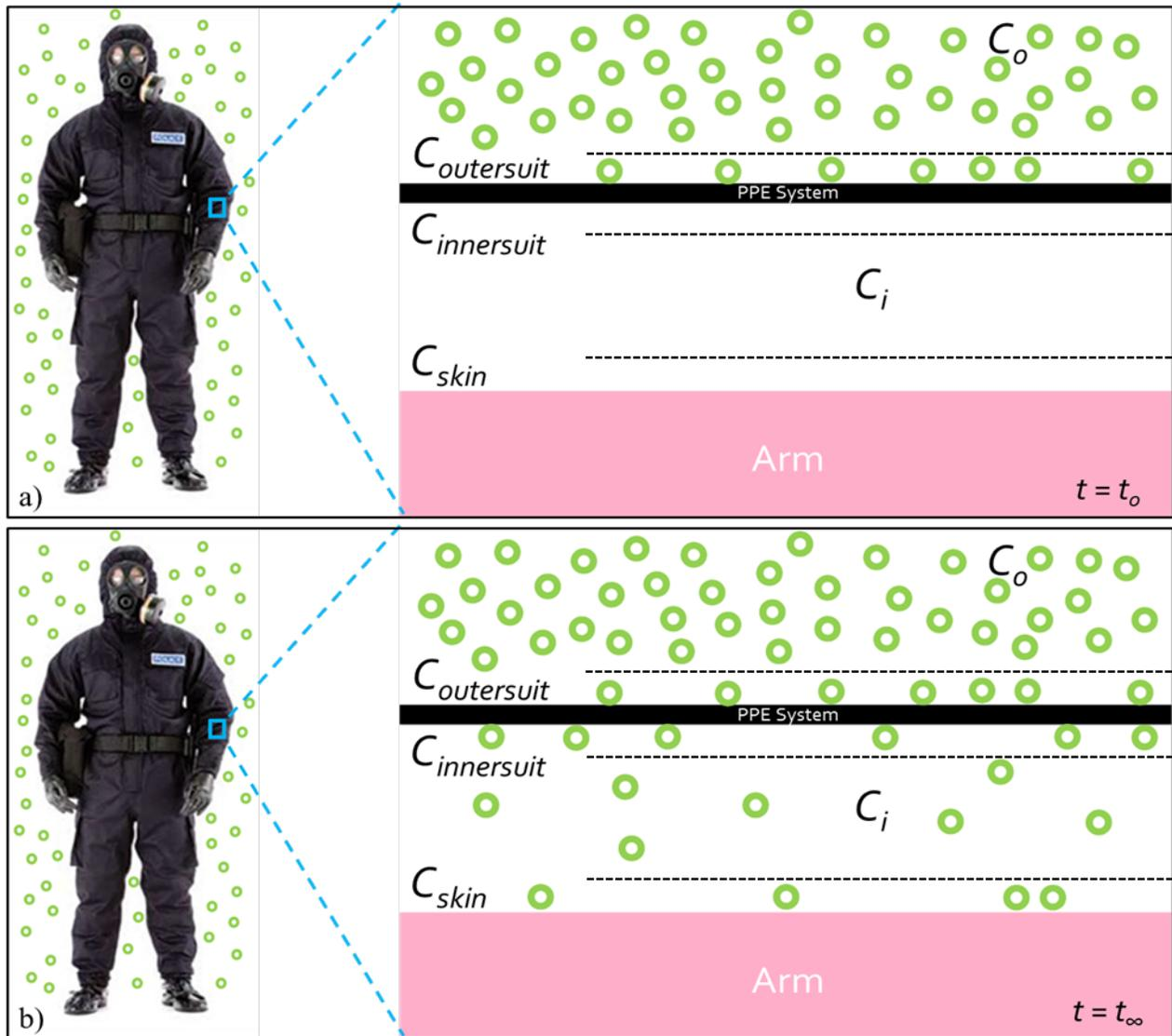
Figure 1: Regional concentration profile at  $t_0$  and  $t_{\infty}$  for an air permeable fabric
