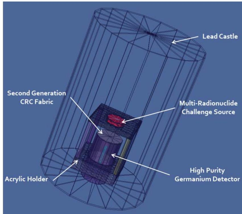
Figure 5: MCNP5 model geometry used to simulate transmittance experimentation
