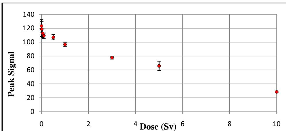
**Figure 3:** Decay curve of the 0.2 μM fluorescein solution
