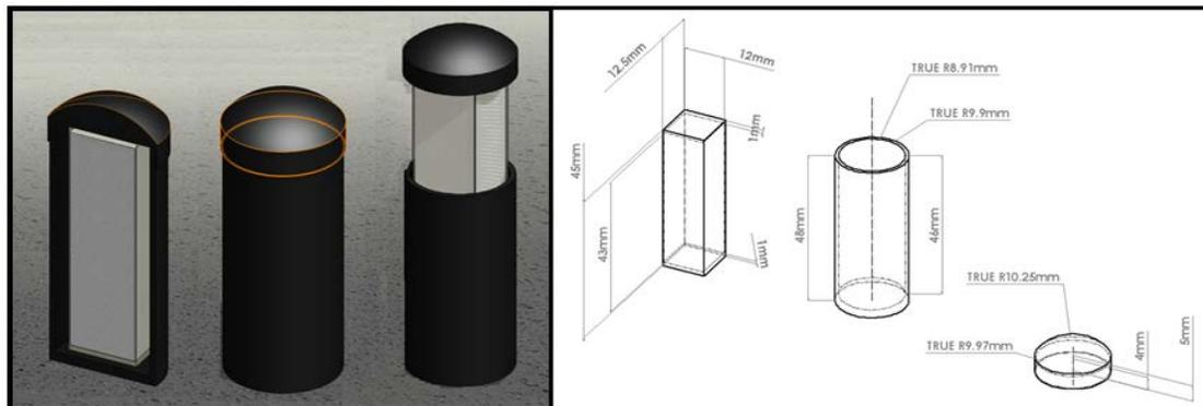
Figure 5: Proposed preliminary design of the fluorescein dosimeter.
