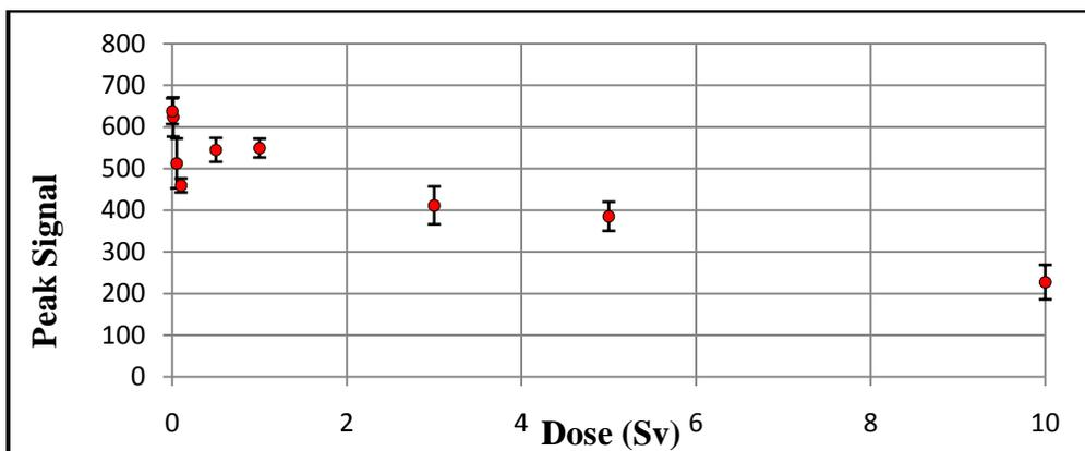
**Figure 4:** Decay curve of the 1.0 μM fluorescein solution
