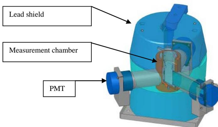
Figure 1. Detector assembly of Hidex 300 SL LSC [7].
