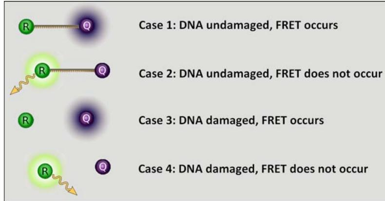
Figure 3 Possible scenarios after the DNA dosimeter is exposed to ionizing radiation.  $R$  represents the reporter molecule and  $Q$  represents the quencher molecule.
