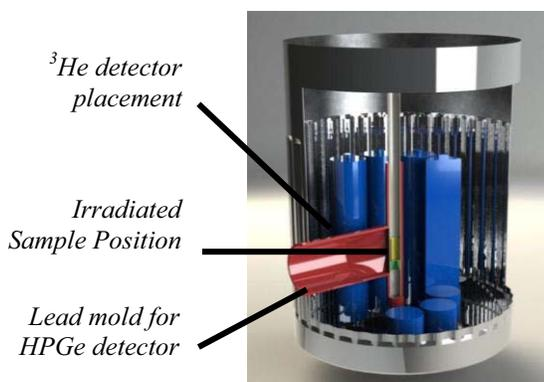
Fig. 1. A Schematic of the DNGC System
