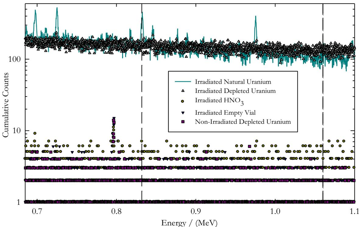
Figure 3: Relative count contributions from depleted & natural uranium, empty vials and the HNO<sub>3</sub> solution.
