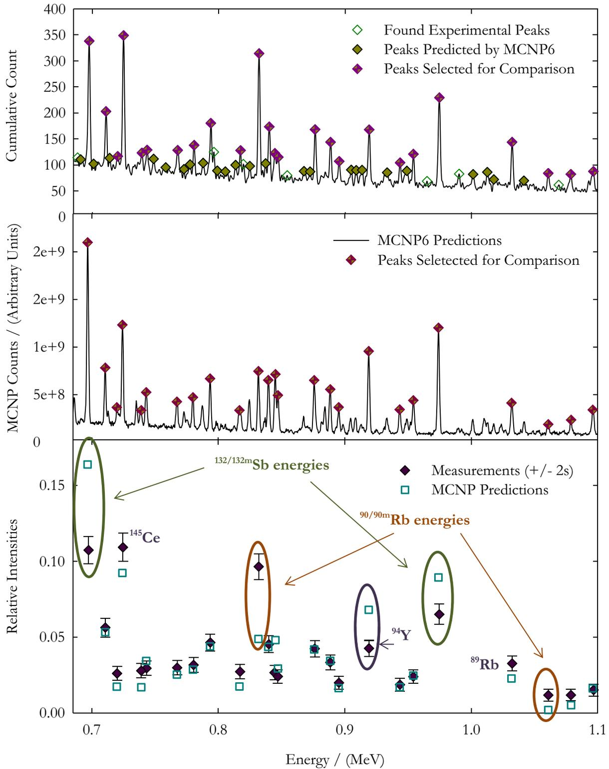
Figure 2: Measured and MCNP6 Simulated Delayed Gamma Count Comparisons
